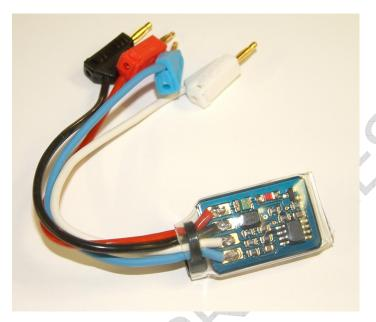
The **inverter** is powered directly from the **bC16**'s external +5v power buss which is available on two of the 2mm patch sockets found on the **bC16** and is connected like so:
